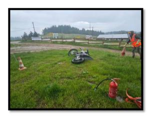
A dedicated way from the track to the quarantine zone/burning zone must always be arranged and kept free from any obstacles in order to allow the extraction a faulty motorbike without any delay.
